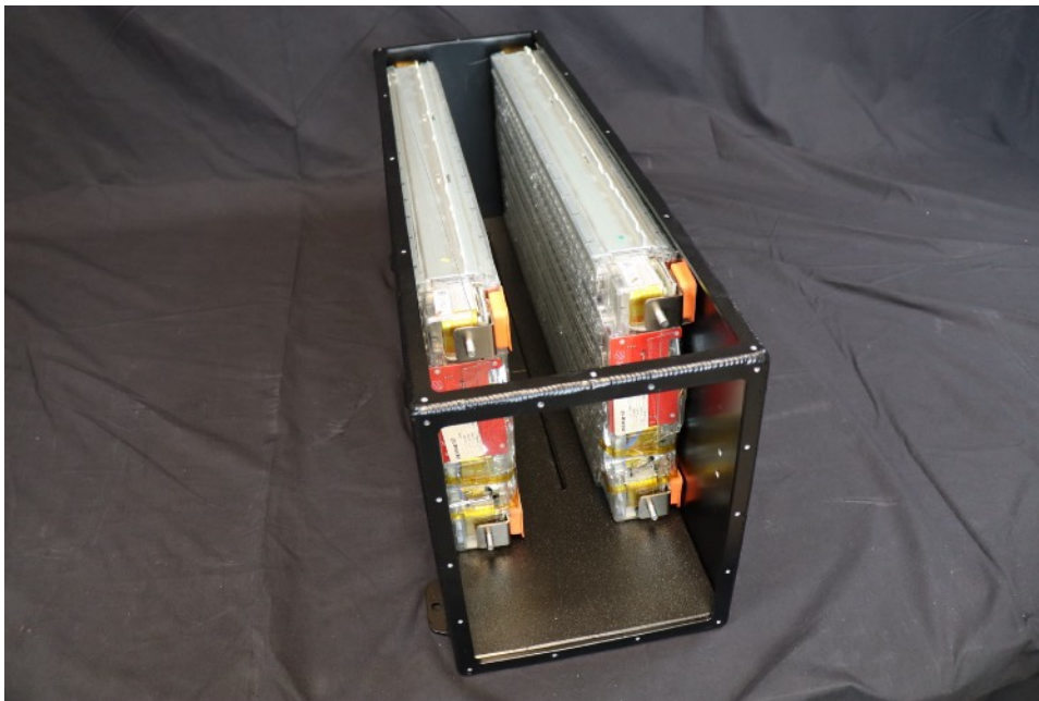
Install rear battery. Note the direction of battery collectors.
