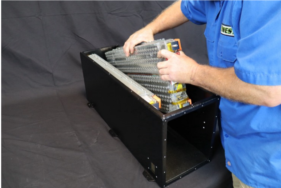
Install rear battery.
