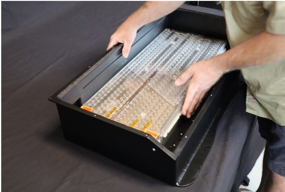
Install first battery module
