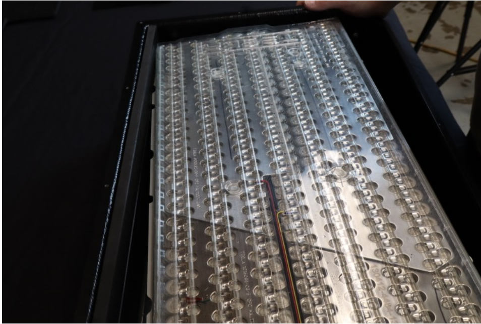
Install second battery module
