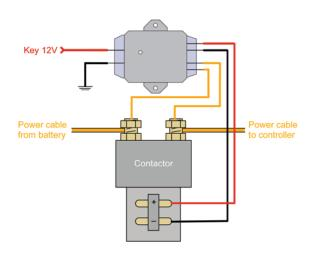
For more complete EV wiring diagrams, please consult the Tech Info section of our website at **www.zeva.com. au**. Electrical connections are made using standard 1/4" spade crimp terminals. There are a total of six connections to make as follows:
