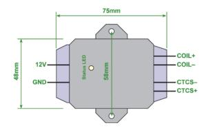
The precharger may be installed in any orientation, and should not require any additional weather protection unless used in marine environments.
