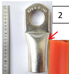
Mark the length to be inserted in terminal about 7/8"
