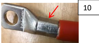
Completed crimp example top to bottom with no gaps
