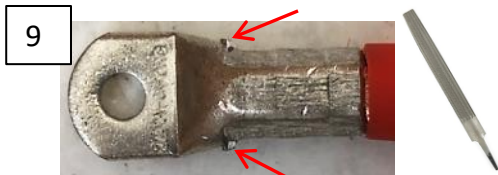
If metal "ears" appear from the crimping process clean them off with a file
