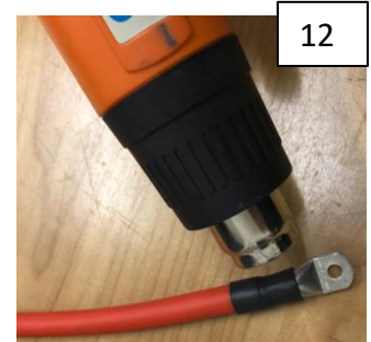
Position the shrink tube clear of the stud section. Apply heat constantly moving the gun around the tube until the glue starts to weep out.
