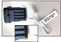
Connect the enable plug into the enable harness connector at the end of the pigtail which is hardwired into the converter.
