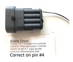
Connector wired correctly? —> Disregard TSB and diagnose using standard procedures. Connector wired incorrectly? —> Proceed to the following repair steps.
