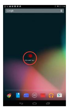
**4.** You can open the app, or plug in the EVCC and it should auto-detect and prompt you to open it with a program from the list. If this is what you choose to do, select FTDI UART Terminal from the list. (you can also check the box to always open with selected program). Once it is open, push the menu button (this differs from android to android).
