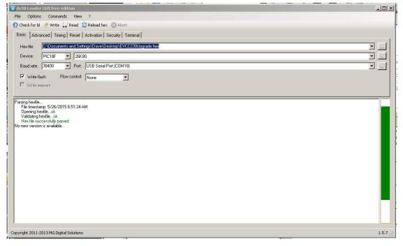
**Upgrade Step 3**: Once the correct parameters are set, click on the "Write" option (just to the right of "Check for bl").
