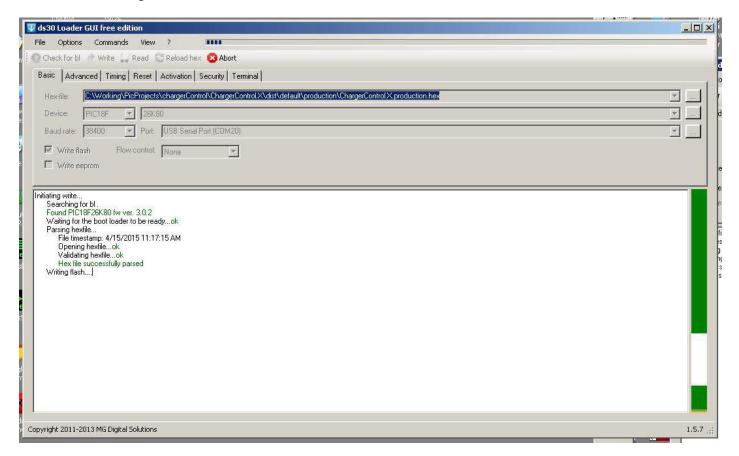
**Upgrade Step 4**: Once the upgrade has completed, it is necessary to exit from the ds0bootloader application, **cycle power** to the EVCC, and start the terminal application.
