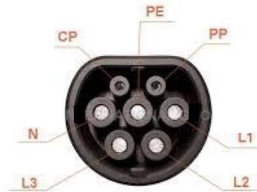
Figure 12 – Face of J1772 Type 2 Socket
