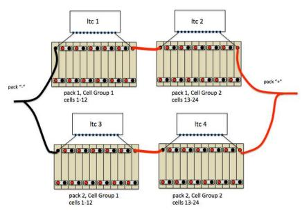
Figure 5 – Two Parallel 24 Cell Packs Wired to the BMS
