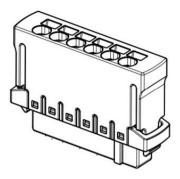
Figure 8 – Harting Push-in Connector
