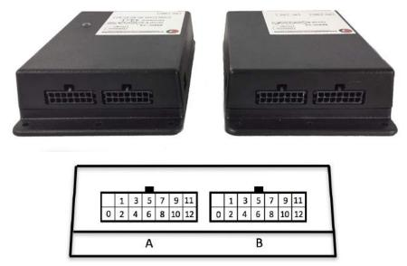
**Figure 11 – Cell Harness Connections**
