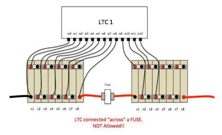
Figure 3 – LTC Wiring Spans A Fuse
