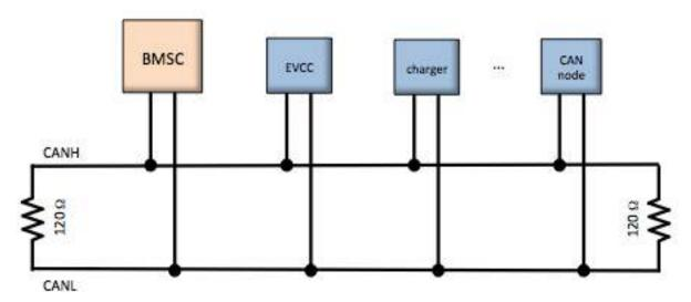
Figure 14 - CAN Network Diagram
