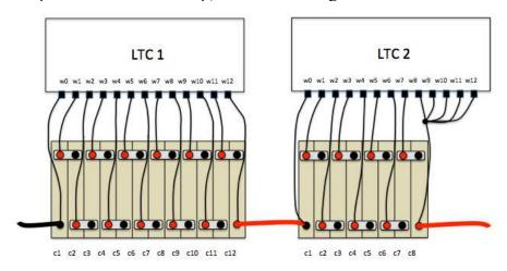
Figure 2 – Cell Group Wiring
