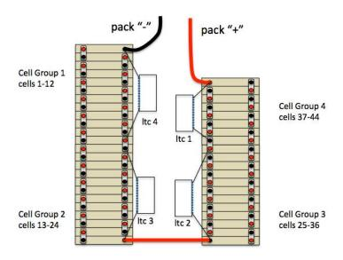
Figure 6 – 44 Cell Pack, LTCs connected where convenient
