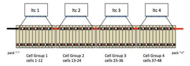
Figure 4 – 48 Cell Pack Wired to the BMS
