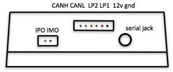
Figure 9 – BMSC System Connections
