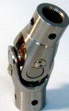
.750-20 SPLINE (201) x .688-34/36 SPLINE (108) Adapts Woodward shaft to the Toyota 600 box. Has one filled or "block" spline; not indexable on the steering box. UA201108..... 90.00
