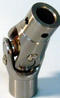
.688-34/36 SPLINE (108) x 3/4 WELD-ON (100) Fits Delphi 600 series box used on Toyota truck. Has one filled or "block" spline; not indexable on the steering box. UA108100 ..... 87.08
